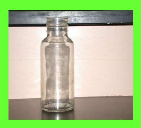
Used to collect large volumes of gas through the use of water displacement
