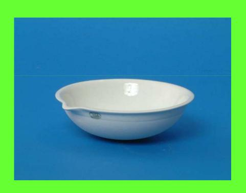
Used to evaporate solutions (evaporate liquid, leaving solid behind)
