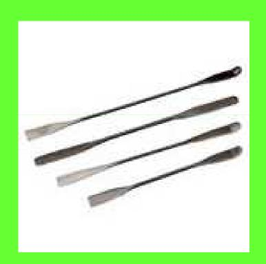
Used to transfer solids from container to container
