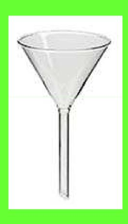
Used to transfer and filter solid particles from liquid solution
