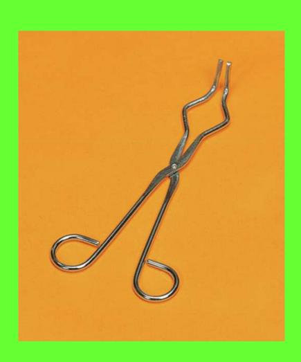
Used to hold and move crucibles and hot glassware
