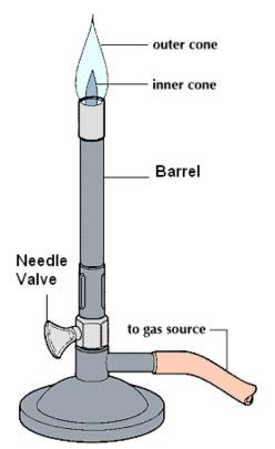
The type of flame is controlled by varying the relative amounts of gas and air entering the barrel. Major adjustments in gas flow are made by turning the handle on the bench gas valve. More precise control is achieved by careful adjustment of the needle-valve screw at the base of the burner. The amount of air entering the barrel is controlled by rotating the barrel to reposition the collar. The rotation causes the collar to cover the air inlet holes to a greater or lesser extent.
